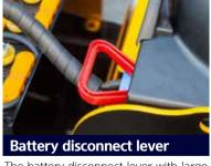
The battery disconnect lever with large handle helps separate the battery connector from the vehicle.
