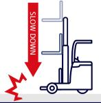
When the forks are being lowered, a down-control valve maintains the controlled speed. The down-safety valve prevents forks from dropping down in case of sudden damage of hydraulic line.
