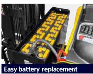
By using the reach out function of the reach cylinder, the battery can be removed, checked, and exchanged easily.
