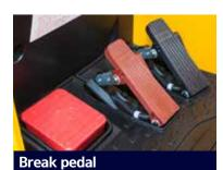
Smoother breaking is assured by the balanced design of the pedal and maintenance costs are lowered as the cover is easily replaceable.
