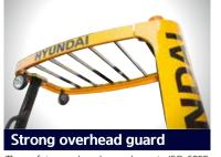
The safety overhead guard meets ISO 6055 and ANSI regulations and protects the operator during hazardous work.
