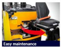
The rotating hood with hinges can be opened up to 105 degrees. So the operator can check and repair the driving device located underneath the seat.
