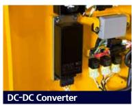
DC-DC converter satisfied with UL & CE prevents from short circuit overload and reverse polarity.
