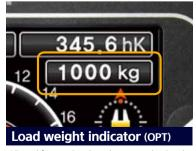
When lifting a load, a change in hydraulic pressure of the lift line is converted to a measurement of weight displayed in real time, and a warning is given at the time of overload.
