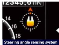
The symbol of the cluster shows the angle of the steering wheel. So the operator can easily predict the direction
