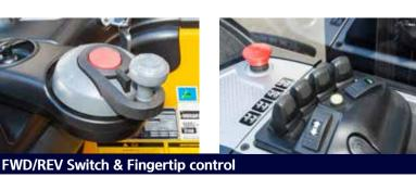
The forward/reverse switch provides the operator with precise and smooth directional control. And responsive fingertips with less energy offer productivity improvement and safety. So the driver can feel less fatigue.
