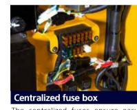
The centralized fuses ensure easy inspection and replacement.
