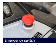
In case of an emergency, the emergency switch is installed to block the battery power supplied to the vehicle to prevent damage and safety accidents.
